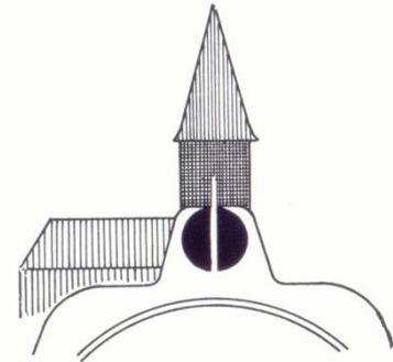
Employ tangent screw [3] to move staff to centre of field of view. By means of focussing knob [7], image is now made to appear sharp.
