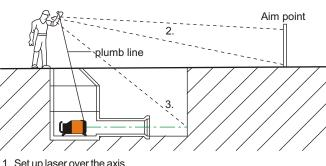
. Set up laser over the axis.
